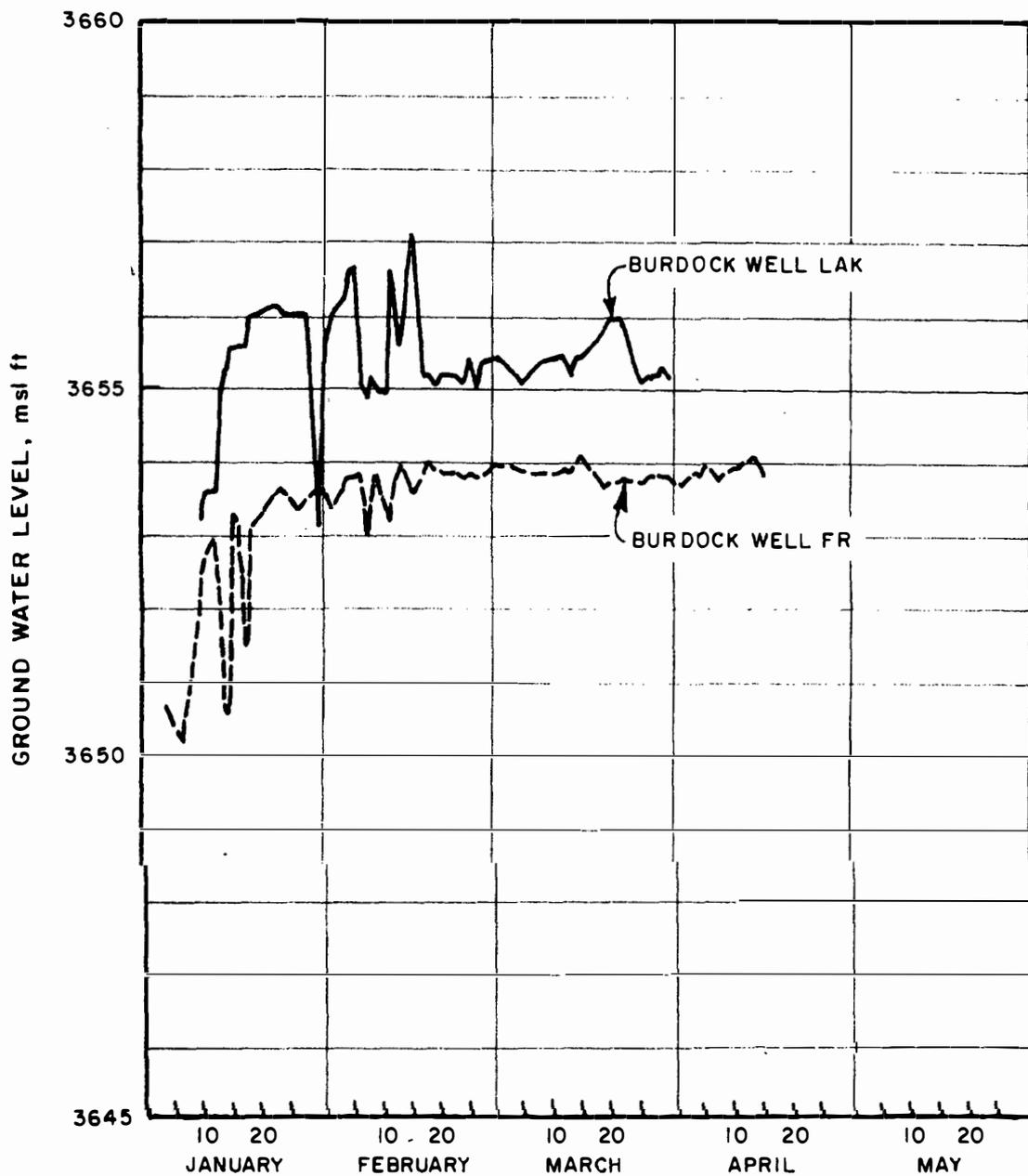
Figure 4 : Hydrographs for Burdock Test Well, January 1 through April 17, 1979
