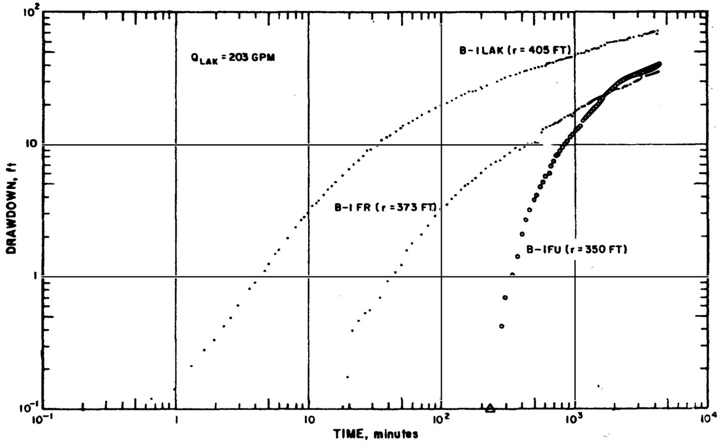
Figure I4 : Logarithmic Graphs of Drawdown for B-1 Observation Well Group, Lakota Aquifer Test
