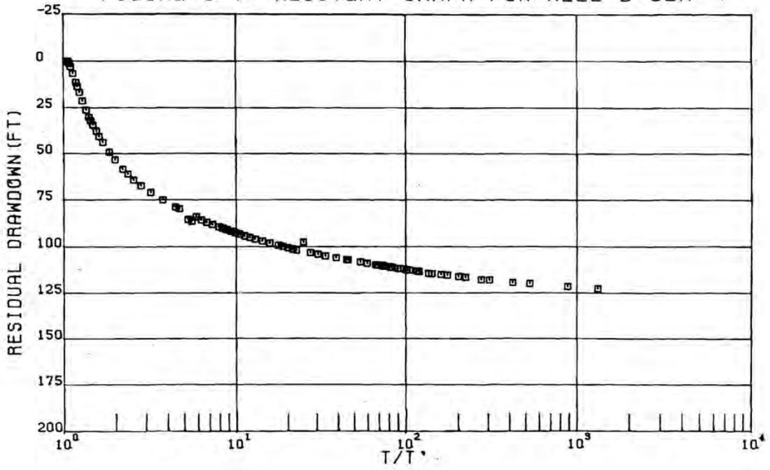
FIGURE C-9: RECOVERY GRAPH FOR WELL D-20LK
