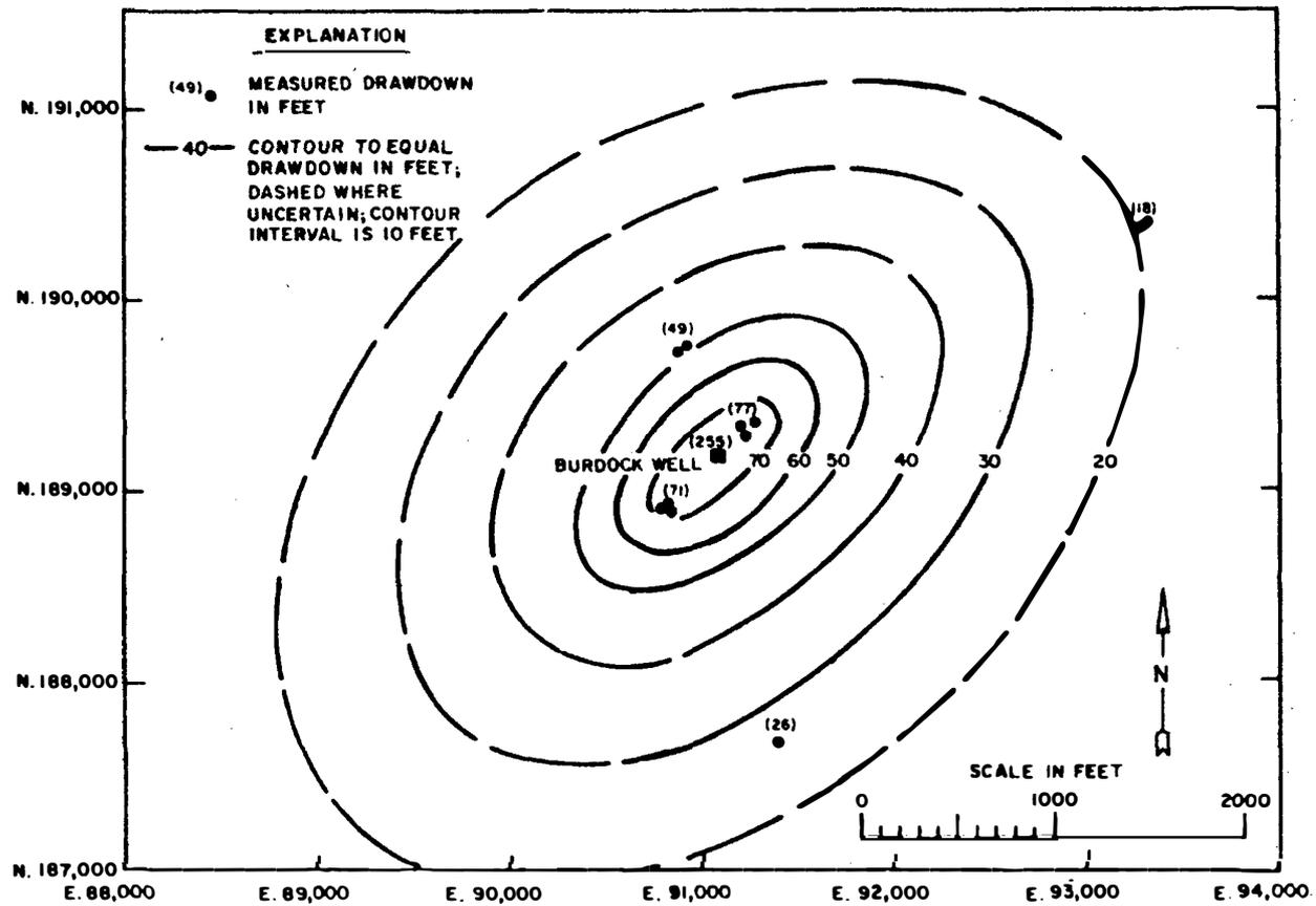
Figure 19 : Drowdown In Lakota Aquifer at End of Lakota Test
