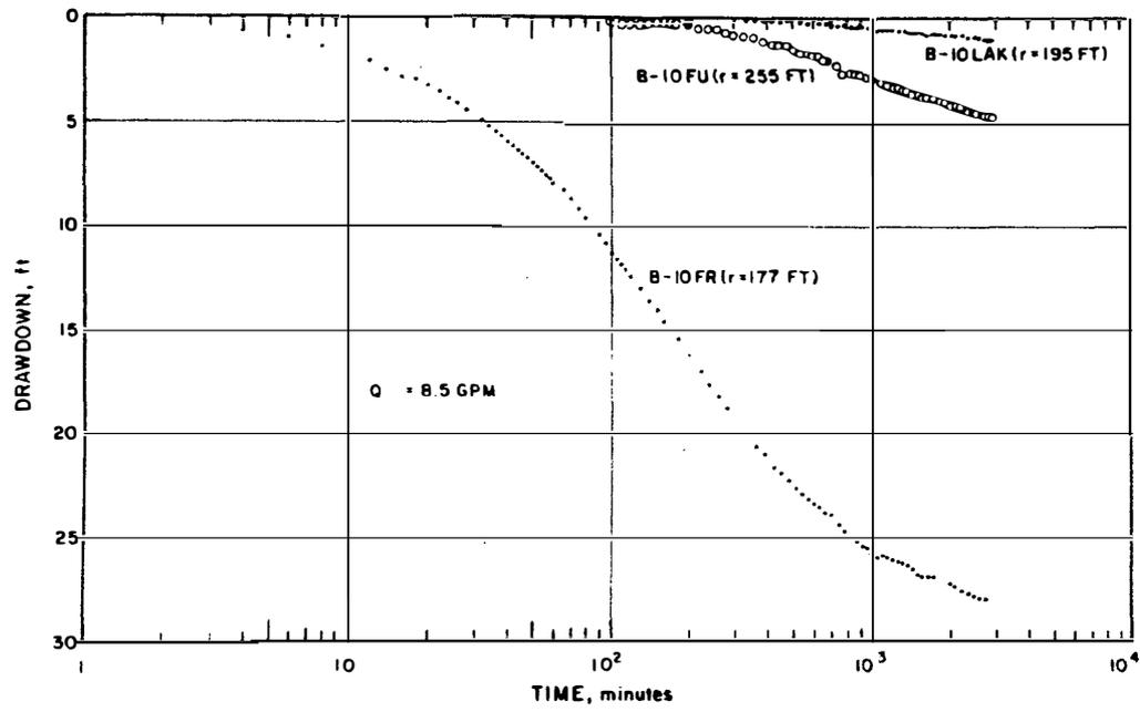
Figure 27: Semilogarithmic Graphs of Drawdown for B-IO Observation Well Group, Fall River Aquifer Test
