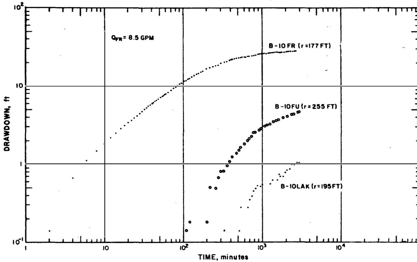
Figure 31: Logarithmic Graphs of Drawdown for B-IO Observation Well Group, Fall River Aquifer Test
